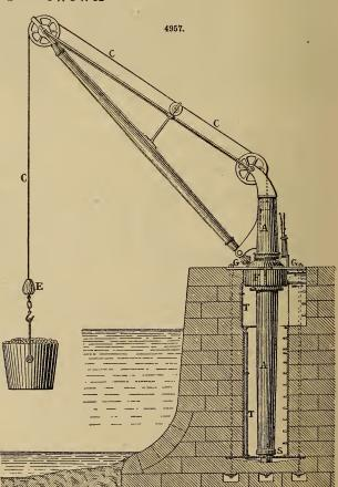
crane is made to revolve. This pinion is worked by a worm and wheel V placed in the counterpoise box H; and two men are sufficient to move round the crane with 60 tons suspended from the extreme point of the jib. In working the crane the men stand upon a cast-iron platform W attached to it a few inches above the level of the ground.
